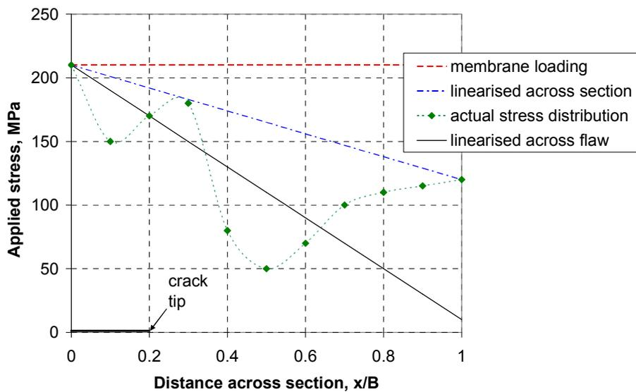
**Figure 1.** Example of stress distribution across a component, showing how it can be idealised for input into a BS7910 fracture assessment.
