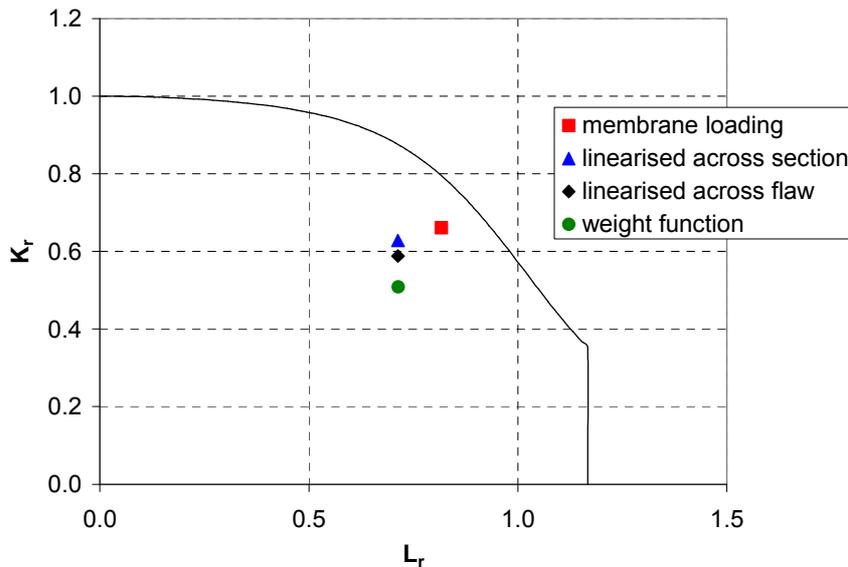
**Figure 2** Example of BS7910 fracture analysis (Level 2) using different types of stress input.
